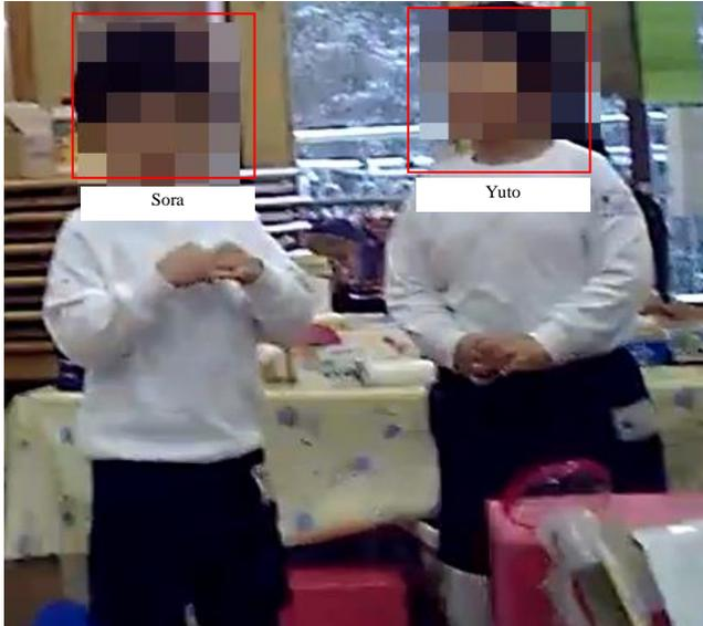
Fig. 2. Face recognition and personal authentication in our system. Recognized faces are illustrated using rectangles. For the protection of personal information, mosaic is attached in the faces and these names are temporary.
